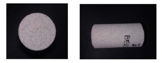
Parameter of Core Berea Stone •Diameter: 24.73mm •Length: 50mm •Porosity: 22.1% •Permeability: 650mD
